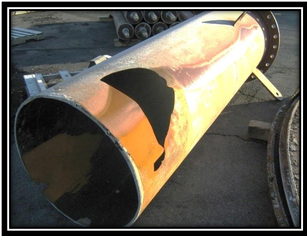
1) Damaged Pipe with Worn Lining
